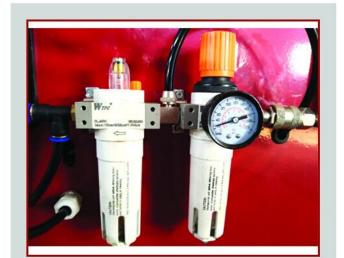
1.0 Mpa high pressure resistance water and oil filter
