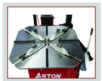
Double wear-resist scribings let the wheel clamps move smoothly. The Stop Block can avoid wheels scratching and also position wheel rim automatically
