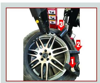
Three-point tire push system will work easier and more efficiently for different tire changes.
