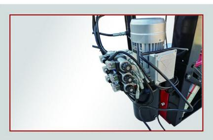
Power hydraulic system works together with electric system, provides much longer service life and a more stable quality than pneumatic system.
