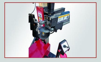
Central column integration 2.0. Hydraulic system makes it more stable, easier to control and creates a higher working rate. Double disc wheel can both lift and press tires. Automatic operation avoids touching or controlling tires by hand.
